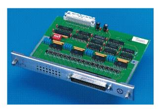
The DI input cards may be indifferently used for reading simple signalizations, double (complementary) signalizations, binary coded analog values and the acquisition of counting (totaling) pulses.
